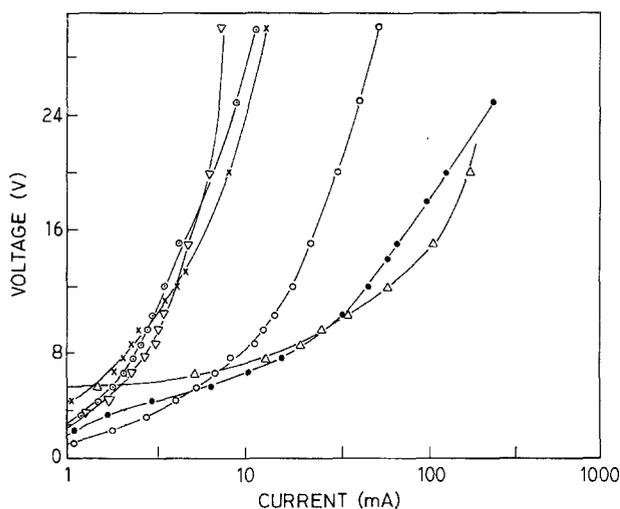
Figure 1  $V-I$  curves of the samples sintered at  $900^{\circ}\text{C}$ .  $\times$ , pure ZnO. ZnO + percentage  $\text{Nb}_2\text{O}_5$ :  $\bullet$ , 0.1%;  $\Delta$ , 0.2%;  $\circ$ , 0.3%;  $\nabla$ , 0.4%;  $\diamond$ , 0.5%.
