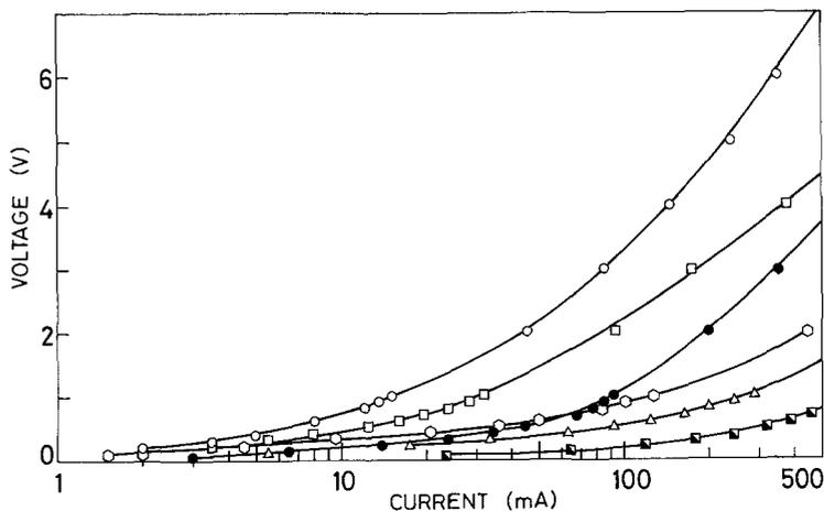
Figure 4  $V-I$  curves of the samples sintered at  $1200^{\circ}\text{C}$ .  $\circ$ , pure ZnO. ZnO + percentage  $\text{Nb}_2\text{O}_5$ :  $\square$ , 0.1%;  $\bullet$ , 0.2%;  $\triangle$ , 0.3%;  $\blacktriangle$ , 0.4%;  $\blacksquare$ , 0.5%.
