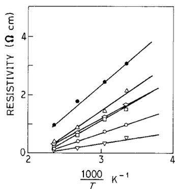
Figure 8 Dependence of resistivity with temperature for samples sintered at 1100°C. ○, pure ZnO. ZnO + percentage Nb<sub>2</sub>O<sub>5</sub>: □, 0.1%; ●, 0.2%; △, 0.3%; ◇, 0.4%; ▽, 0.5%.
