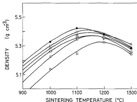
Figure 7 Plot of variation of density as a function of sintering temperature for the ZnO- $\text{Nb}_2\text{O}_5$  system.  $\circ$ , pure ZnO. ZnO + percentage  $\text{Nb}_2\text{O}_5$ :  $\square$ , 0.1%;  $\bullet$ , 0.2%;  $\triangle$ , 0.3%;  $\diamond$ , 0.4%;  $\nabla$ , 0.5%.
