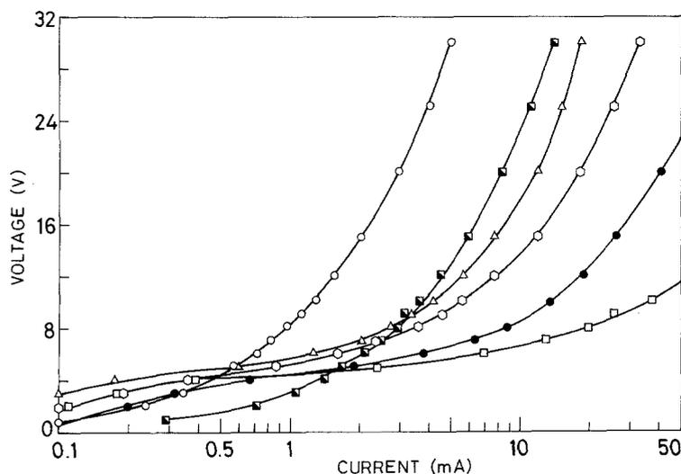
Figure 2  $V-I$  curves of the samples sintered at  $1000^{\circ}\text{C}$ .  $\circ$ , pure ZnO. ZnO + percentage  $\text{Nb}_2\text{O}_5$ :  $\diamond$ , 0.1%;  $\square$ , 0.2%;  $\bullet$ , 0.3%;  $\Delta$ , 0.4%;  $\blacksquare$ , 0.5%.
