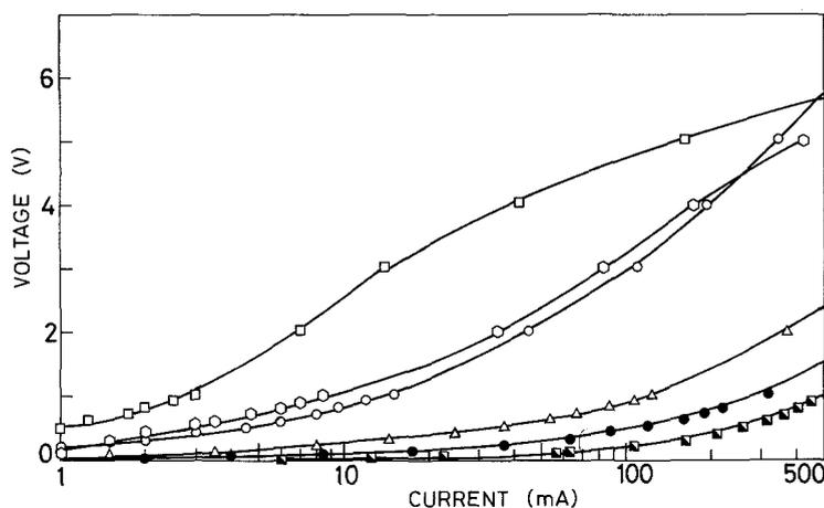
Figure 5  $V-I$  curves of the samples sintered at  $1300^{\circ}\text{C}$ .  $\circ$ , pure ZnO. ZnO + percentage  $\text{Nb}_2\text{O}_5$ :  $\square$ , 0.1%;  $\bullet$ , 0.2%;  $\triangle$ , 0.3%;  $\blacktriangle$ , 0.4%;  $\blacksquare$ , 0.5%.
